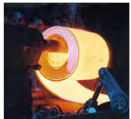
1.5.3 Coilbox in the Bochum hot strip mill: The Coilbox is located between the roughing mill and the finishing stands. The transfer bars from the roughing mill are rapidly coiled and then subsequently uncoiled and fed at a lower speed to the finishing stands. Forming a transfer bar into a coil dramatically reduces radiant heat loss and produces a virtually uniform temperature in the uncoiled transfer bar as it enters the finishing stands.
