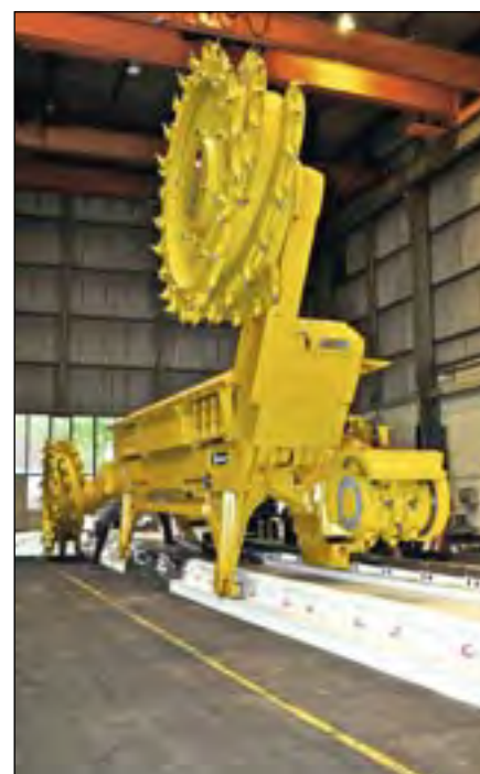
3.3.3 Disk shearer produced by the mining supply company Eickhoff Maschinenfabrik in Bochum
